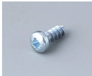
A0308031 Self-tapping screws 3 x 8 mm (PZ1)
