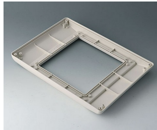
B4046707 Bottom part L flat, version I ABS (UL 94 HB) off-white RAL 9002 275x195x26.5mm IP 54 opt.
