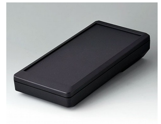
A9075119 DATEC-MOBIL-BOX L, Vers. I ABS (UL 94 HB) black RAL 9005 252x121x50mm IP 65 opt.
