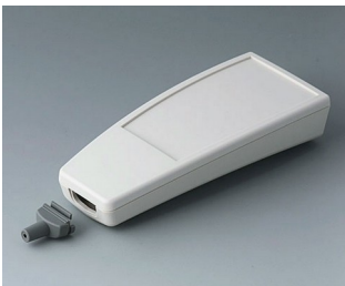
A9068147 SMART-CASE XL, Vers. V ABS (UL 94 HB) off-white RAL 9002 168x74.4x35.4mm IP 65 opt., IP 40
