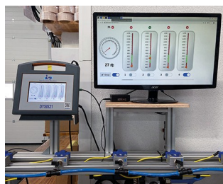
Monitoring system for cleaning nozzles
