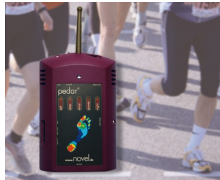
Dynamic pressure measuring between foot and shoe
