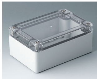
C7012014 IN-BOX ABS/PC (UL 94 HB) light grey RAL 7035 122x82x55mm IP 66, IP 67, IK 07
