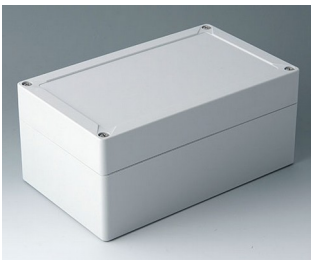
C7020061 IN-BOX ABS (UL 94 HB) light grey RAL 7035 202x122x90mm IP 66, IP 67, IK 07
