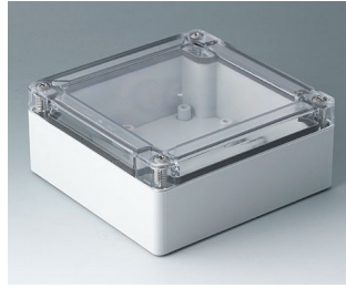
C7013035 IN-BOX PC light grey RAL 7035 124x122x55mm IP 66, IP 67, IK 08
