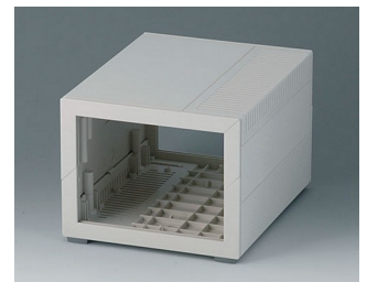
B2213207 MEDITEC E 160, without handle bar ABS (UL 94 HB) off-white RAL 9002 160x200x124mm IP 40
