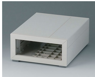
B2213017 MEDITEC E 160, without handle bar ABS (UL 94 HB) off-white RAL 9002 160x200x74mm IP 40
