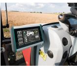
ISOBUS terminal for tractors and self-propelled machines
