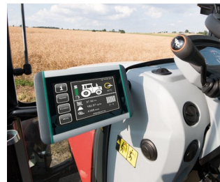
ISOBUS terminal for tractors and self-propelled machines
